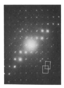
FIGURE 1: a) Electron micrograph taken at 110 K. A diffraction pattern (b) taken from such an area indicates the presence of both the high and low temperature forms.
